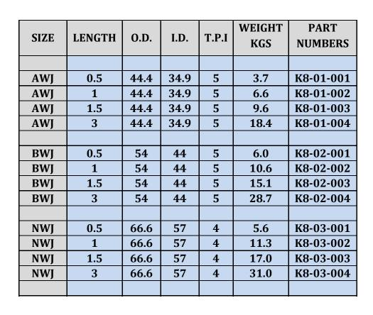
ALL AMKO DRILL RODS ARE MANUFACTURED FROM SEAMLESS CARBON STEEL TUBES , WHICH HAVE EXTREMELY HIGH MECHANICAL PROPERTIES. THE STRAIGHTNESS OF THE TUBES ARE BETTER THAN 1 IN 2000 MM.
